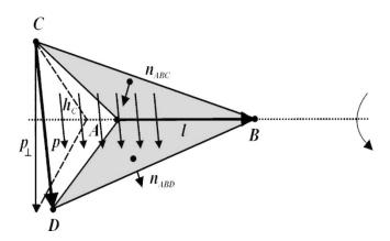
The figure shows an edge-based basis function. The vector variation is perpendicular to the base edge AB (or  $\bar{l}$ ). The vector of the edge CD (or  $\bar{p}$ ) defines the basis function. Within a tetrahedron, the basis function is a constant field given by
