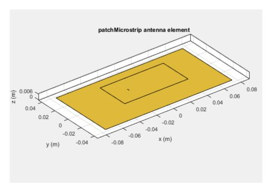
To make the antenna lie on the Y-Z plane, rotate it by 90 degrees about the Y-axis. The rotation follows the standard right-hand rule.
