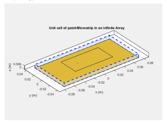
The Antenna Toolbox infinite array is located in the X-Y plane. Unit cells consisting of antennas with ground planes are also located in the X-Y plane. For antennas used as unit cells, such as the one in this example, you ignore the value of the Tilt property.
